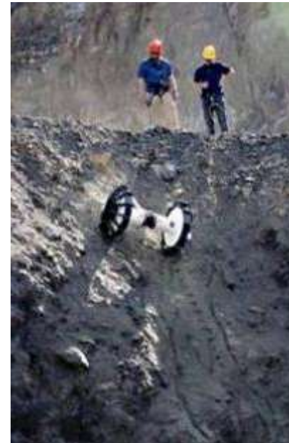
Rappelling a cliff with AXEL robot
