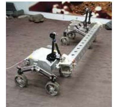
Cooperative beam transport
